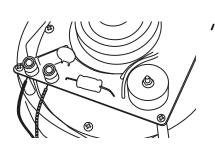
4. Insert the speaker installation tool into two of the screw access holes on the speaker. Carefully place the speaker in the flange; rotate slightly until the speaker surface is even with or slightly recessed into the surface of the flange. While exerting upward pressure, use the tool to rotate the speaker COUNTER-CLOCKWISE (left). This will engage the QM SAFETY-LOC clamps on the back of the flange. Remove tool and tighten the four clamp screws on the speaker. **CAUTION:** do not over-tighten.
